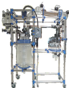
Reactor with horizontal condenser
