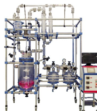
Reactor with PLC automatic system
