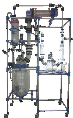
Reactor with rectification column system
